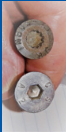
Fig. 6 Left: Screws attaching striker to door sill: I use stainless countersink Hex (6-point, 5mm head) screws as they hold the 5mm tool much better than the 12-point OEM screws. The stainless 6-point screw drives do not get burrs on the drive flanks and over time get so nasty looking. *McMaster 5-pack PN# 93395A414 ($6.89.)
