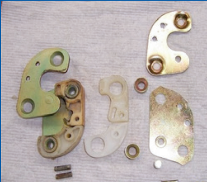
Fig. 1. Driver striker with two pins punched out and the outer plate rotated on the riveted-on striker bar. Then one can remove the two plastic parts. On the right side is another striker with each plate separated.
