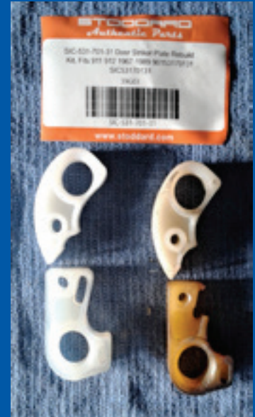
Fig. 2. The new STODDARD striker kit with new white plastic pieces seen here alongside the old parts.
