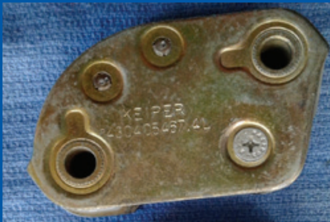
Fig. 1. My striker proved too difficult to punch out the striker bar as it peened over on the back side. I VERY CAREFULLY used a small then larger drill bit slightly larger than the peened over striker bar end, as I did not have the end long enough to re-peen the striker bar end over again, so I drilled into the striker bar with a 5/16" drill, 3/8" deep. Then I tapped it with a 10/32" tap. I then used a counter sink tool to flare out the striker bar end for a countersink machine screw. After cleaning and drying, I installed the new plastic parts then installed a NAS grade 10-32 countersink machine screw and also installed the two alignment pins. Slowly snug the counter sink screw and tap in the pins and lastly tighten the countersink screw. (Any grade 8.8 or better countersink screw will work fine.) The striker's two M8 mounting screws are installed on the door sill and now the unit as a whole is very strong.
