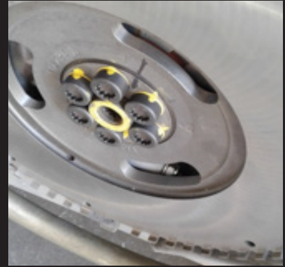
Fig.9. Lightweight flywheel with ARP reusable 12 point cap screws.
