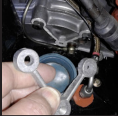
Fig. 8. Cutting off the in-the-way air pump mount casting for 911s.
