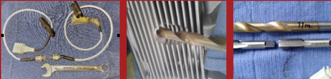
Fig.4.5.6. Enlarged the machined C.H.S (Cylinder Head Temp. Sensor) from 10 mm to the 12 mm for more reliable and less expensive late 993 12mm sensor
