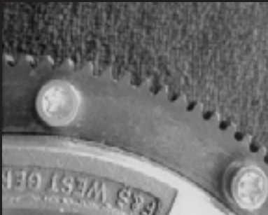
Fig.10. Fully threaded Clutch-flywheel TORX cap screws
