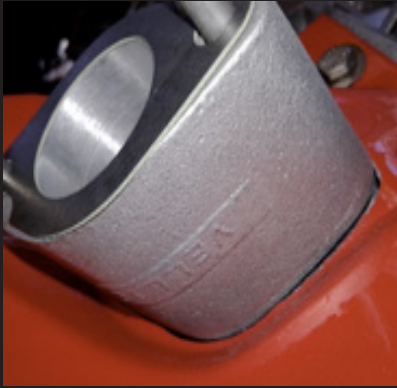
Fig.7. Aluminum Injector intakes 40 mm ported
