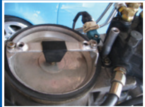
CIS AIR METER white connector. Later one with push wire to release.
