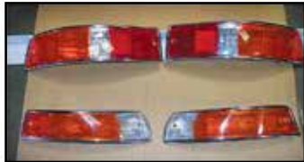
• 1965-68 911 912 light assemblies reconditioned front and rears with new lenses
