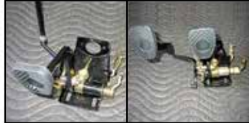
• Reconditioned pedal assembly 1965-1983
