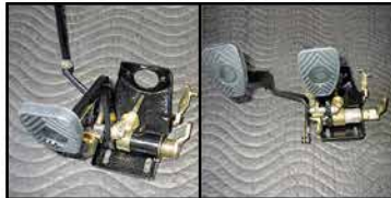
• Reconditioned pedal assembly 1965-1983
