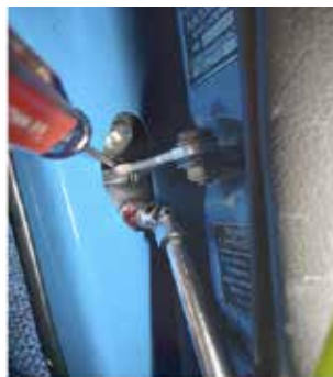
6 mm universal socket & screwdriver to align plates away from Arrestor Arm.
