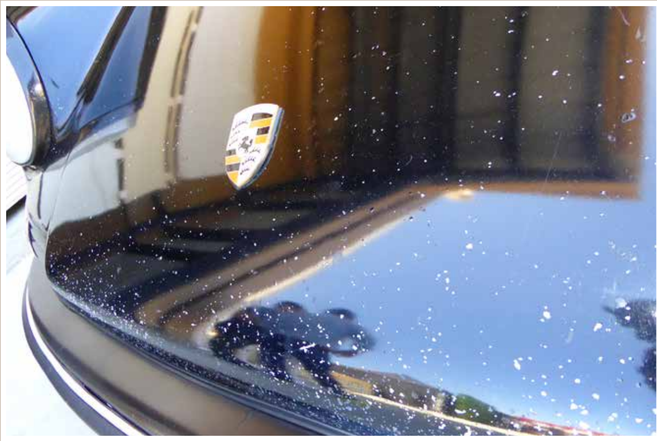
Road rash as seen at Luft 5.
