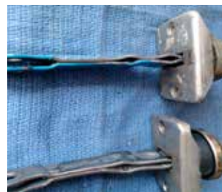
Early Door Supports, worn out.
