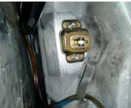
1987 inside door with my modified new Reinforcement Kit and type 964 Door Stop installed.
